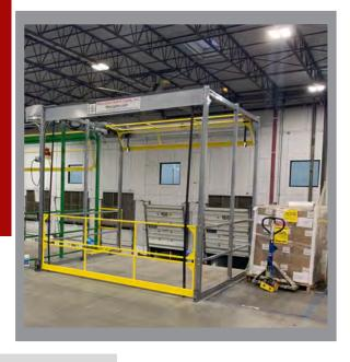
The Roly® Total Control Access (TCA) pallet drop safety gate protects employees working on elevated pallet drop areas, ensuring the ledge is always guarded. The TCA is a power operated, dual-gate system but the gates don't operate in tandem; instead when one gate is opening or closing the other stays fully closed and is prevented from opening until the other fully closes.
