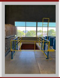
Mezzanine Safeti-Gates invented the first dual-gate safety system, the Roly® mezzanine safety gate, over 40 years ago. We continue to focus on providing fall protection solutions for pallet drop areas on elevated work platforms in manufacturing, material handling and distribution facilities.
