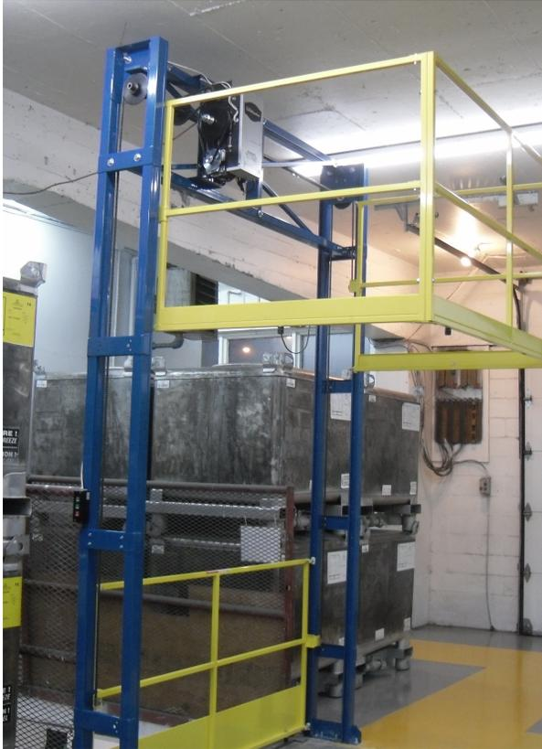
*A Tri-Side Safety Gate model with power operation and photo eyes provides safety for employees and efficiency in the facility.*
