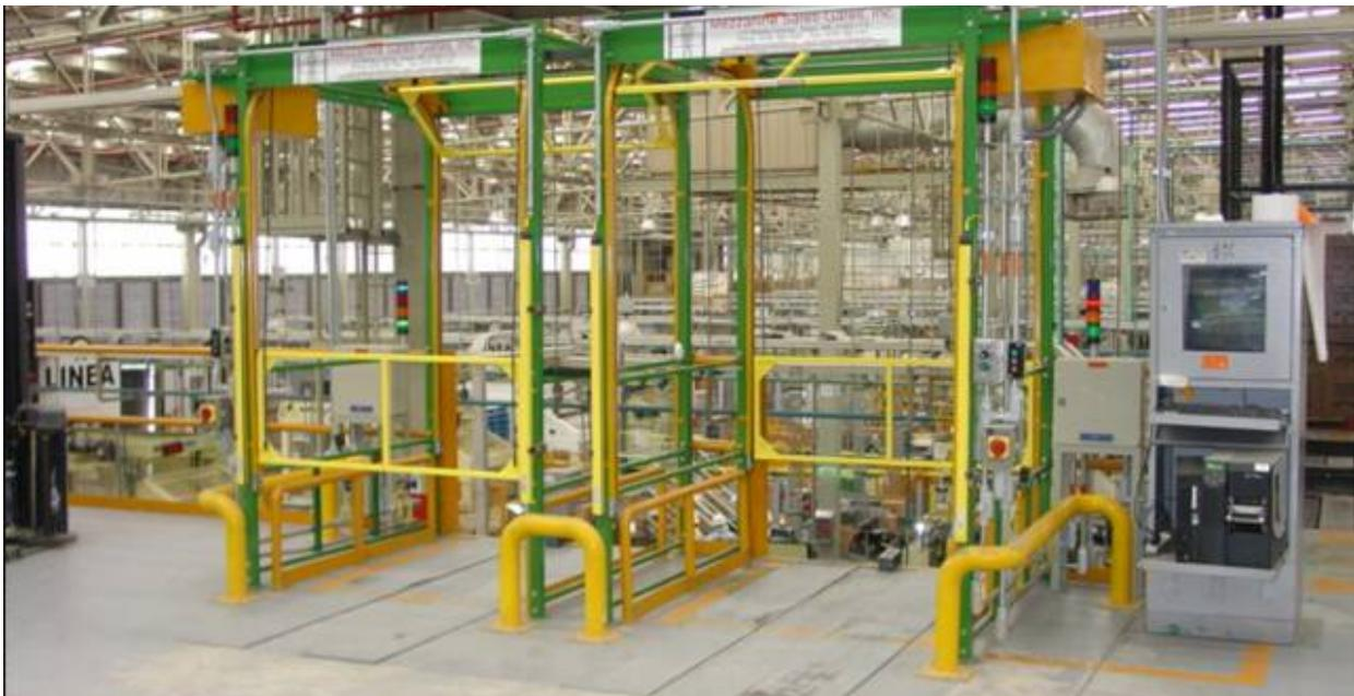
*Two Roly safety gates feature power operation with stations for push-button operation. A fork-lift truck is able to open the safety gates from below with a radio frequency remote.*
